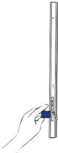
USB card can only be inserted in one orientation. Force to insert the card may in result of damage.
