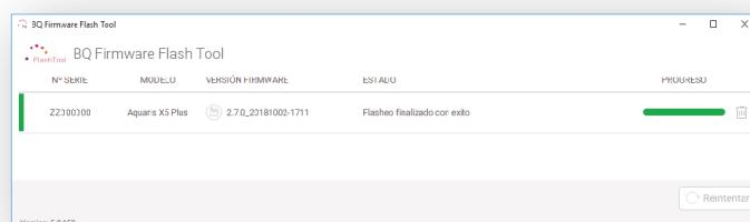
7. The device automatically reboots with the new firmware version installed and ready to go. This first reboot process after installing the new firmware may take longer than a regular reboot.
