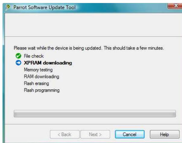
6. When the **Parrot Software Update Tool** reaches the “XPRAM downloading” step, plug in the car kit’s power supply.
