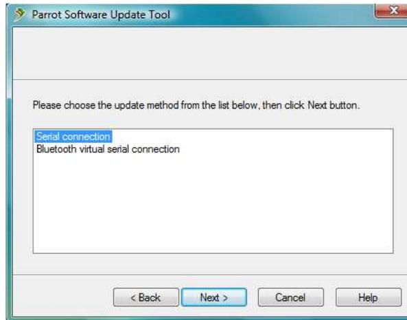
5. Select the COM port on which you have connected the serial cable and click **Next**.
