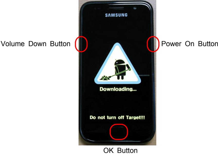
4. Connect the Handset to PC via Data Cable. Make sure ID:COM box highlighted yellow that the handset is connected to the PC.
